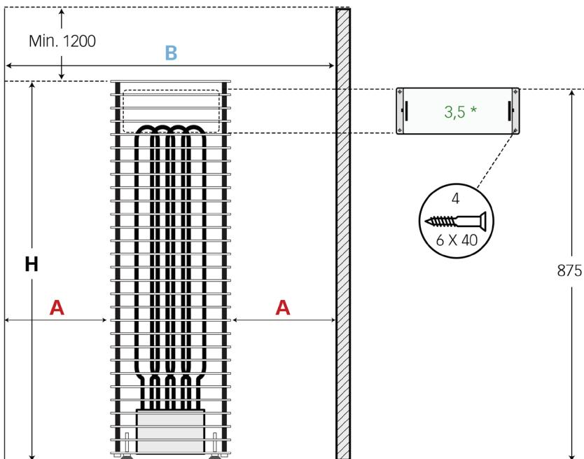
\* CLIFF 3,5 is attached to the wall with a special bracket
